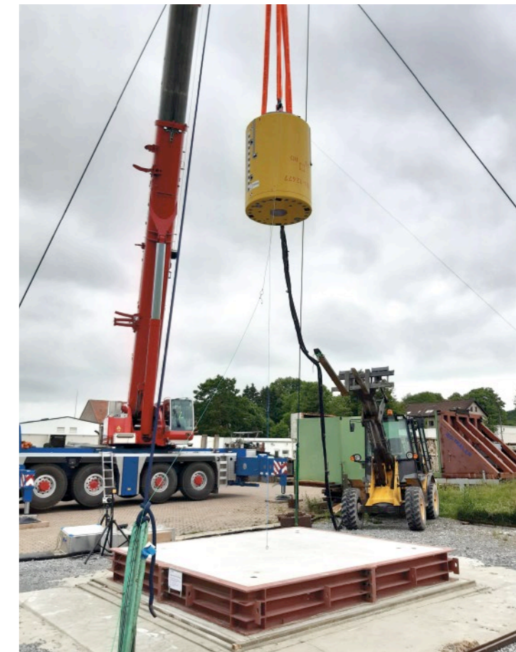
Quality assurance: Container type testing (Photo: GNS Gesellschaft für Nuklear-Service mbH)
